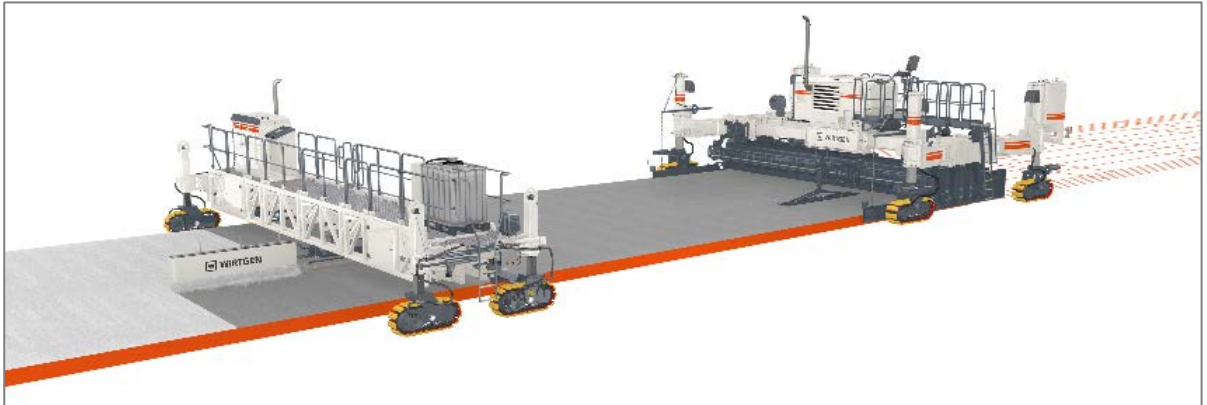
Figure 24: Typical slip-form concrete paving machine operation (from Wirtgen)
